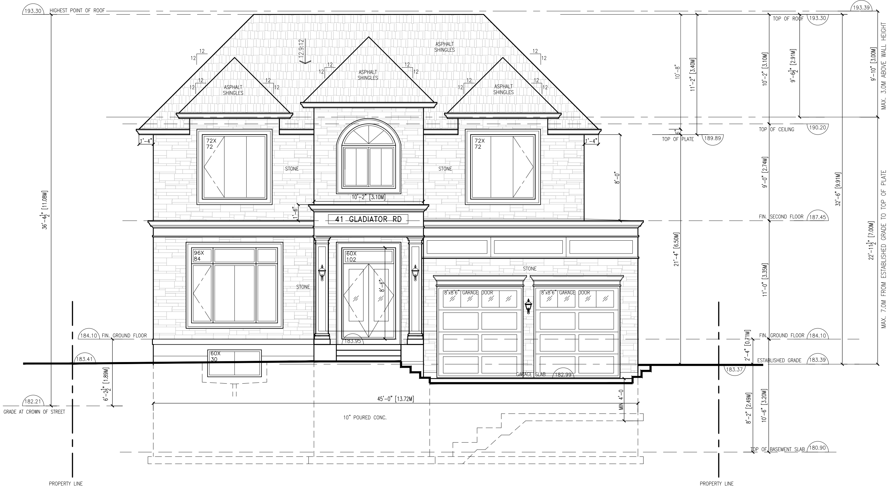
FRONT (WEST) ELEVATION SCALE: 3/16"=1'-0"
