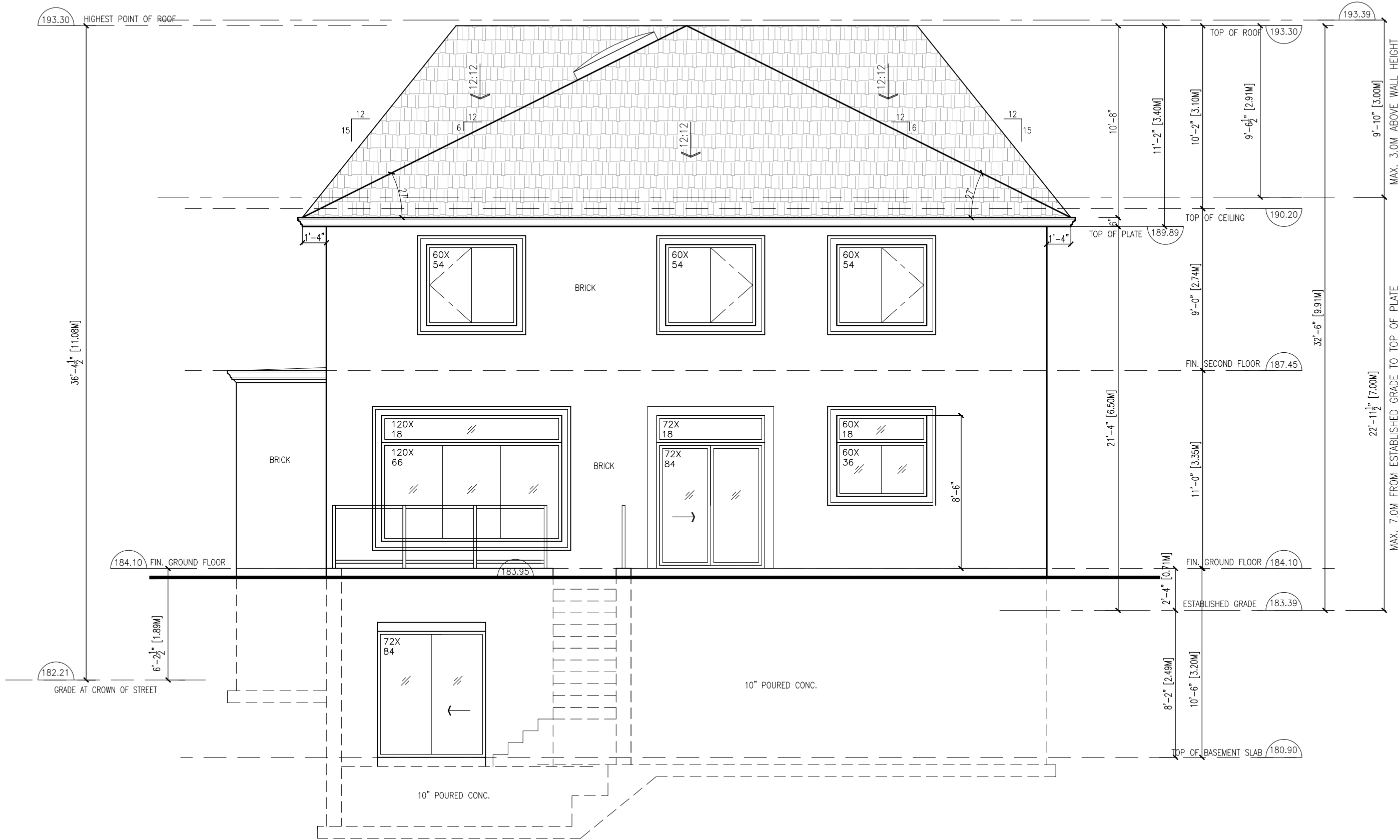
REAR (EAST) ELEVATION SCALE: 3/16"=1'-0"
