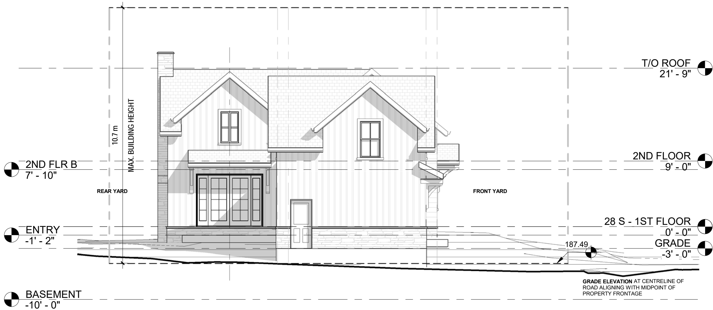
1 28 STATION - WEST ELEVATION 1/8" = 1'-0"
