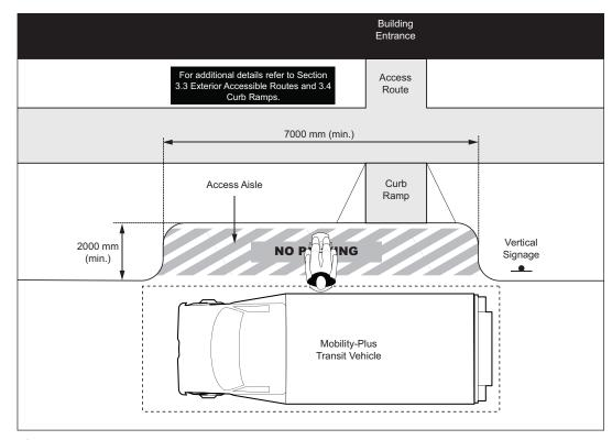
Figure 27: Passenger Loading Zone - Plan View
