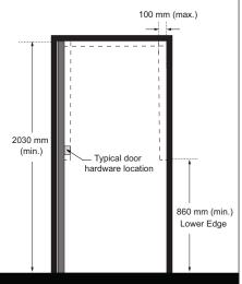
Figure 37: Clear Width of Doors - Plan and Elevation Views
