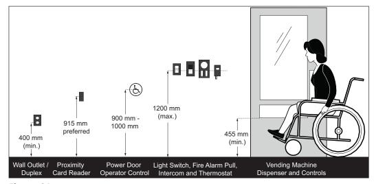
Figure 64: Control Mounting Heights - Elevation View
