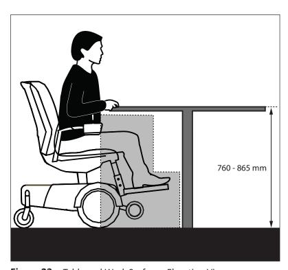
Figure 23a: Table and Work Surface - Elevation View
