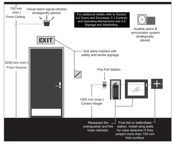
Figure 68: Fire Safety and Evacuation Features - Elevation View
