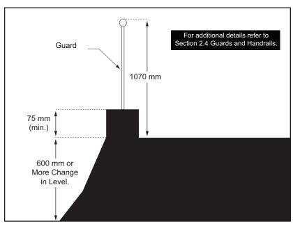
**Figure 9:** Guard Where Level Change is More than 600 mm Adjacent to Ramp Surface - Section View
