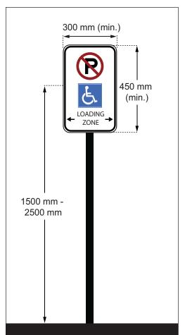
**Figure 28:** Passenger Loading Zone Vertical Signage
