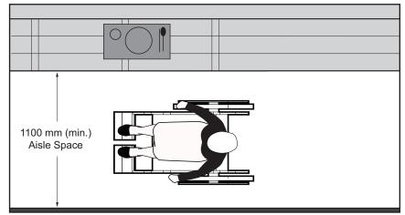
Figure 80b: Aisle Width - Plan View
