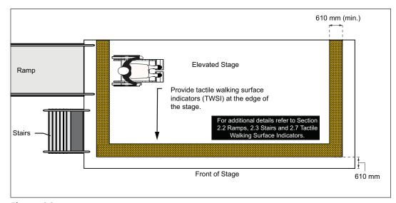
Figure 96: Elevated Platform or Stage - Plan View
