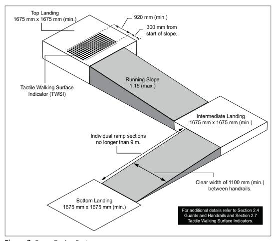
Figure 3: Ramp Design Features
