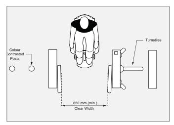
Figure 38: Accessible Controlled Gate
