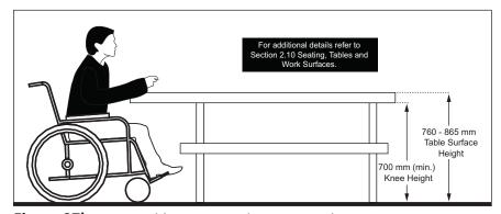
Figure 97b: Picnic Table Design and Features - Elevation View
