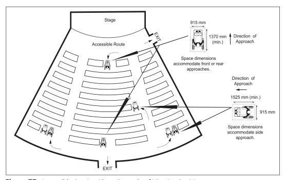
Figure 77: Accessible Seating Plan - Example of Viewing Positions
