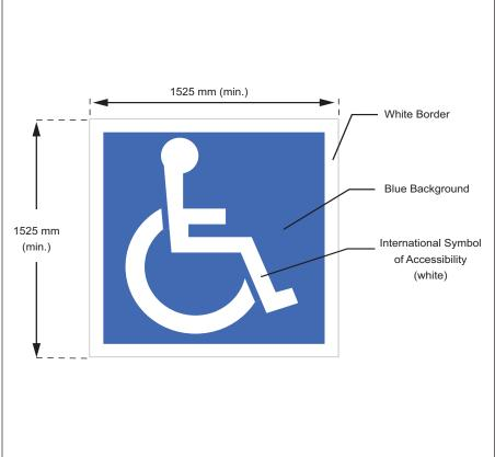
Figure 26: Accessible Parking Pavement Markings
