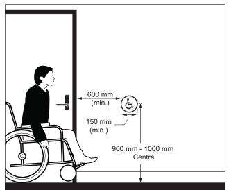
Figure 40a: Circular Push Button - Elevation View
