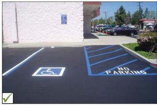
Locate accessible parking space as close as possible to accessible entrance, with accessible route integrated.
