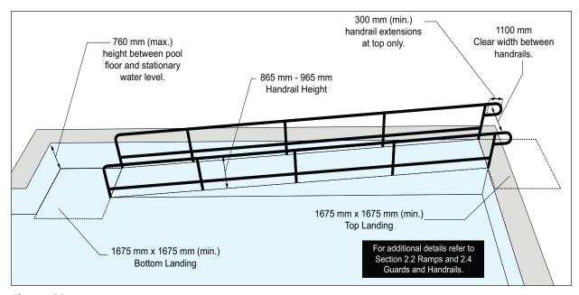
Figure 89: Sloped Entry or Ramp to Swimming Pool
