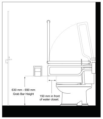
Figure 56b: Fold Down Grab Bars - Elevation View
