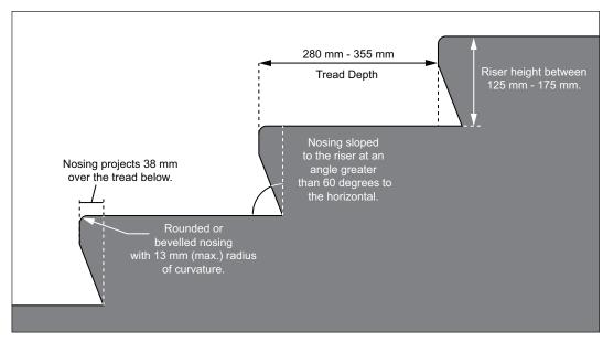
Figure 10: Stair Design Features - Section View
