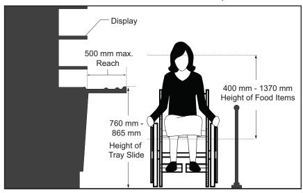
Figure 80a: Food Displays and Tray Slides - Section View
