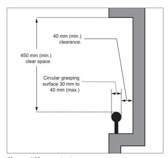
**Figure 13b:** Handrails in Recessed Area - Section View
