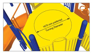
Figure 102: Turning Space - Plan View
