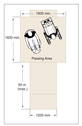
**Figure 29b:** Reduced Clear Width and Required Passing Area
