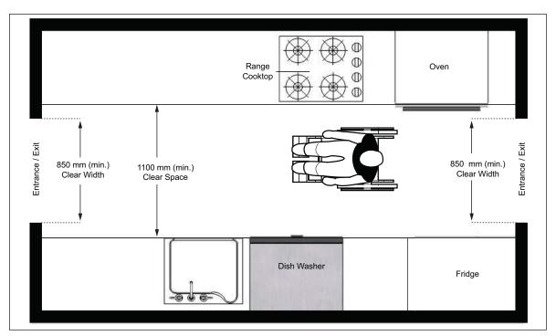
Figure 81: Pass-Through or Galley Kitchen - Plan View
