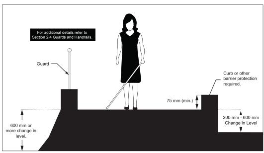
Figure 31: Changes in Level - Section View
