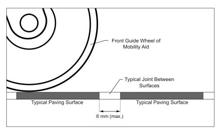
Figure 1: Joints Between Surfaces - Section View
