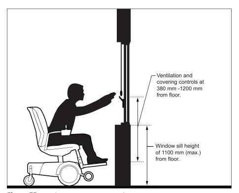
Figure 75: Window Design Features - Elevation View
