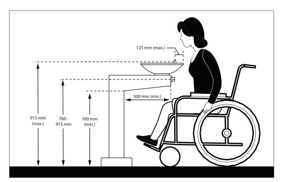
Figure 19: Fountain Design and Layout - Elevation View
