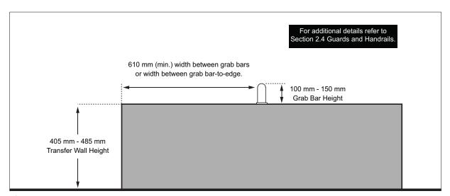
Figure 91: Transfer Wall - Elevation View
