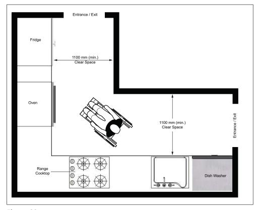
Figure 83: L-Shaped Kitchen - Plan View
