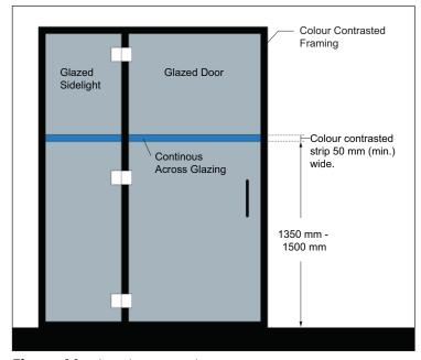
Figure 44: Glazed Doors - Elevation View
