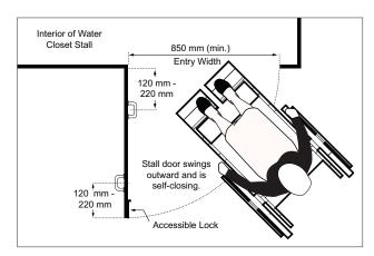
Figure 52: Water Closet Stalls Door Features
