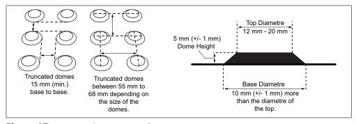
Figure 17: Truncated Dome Specification
