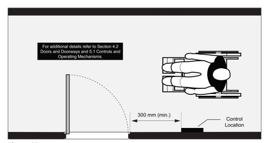
Figure 67: Proximity Card Reader Location - Plan View
