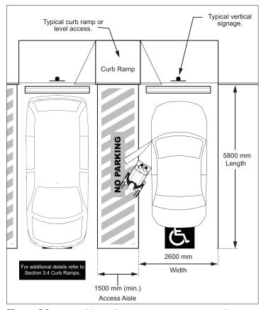
**Figure 24:** Accessible Parking Space Dimensions - Plan View
