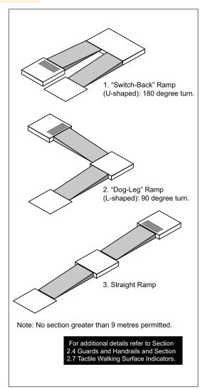
Figure 5: Typical Ramp Configurations
