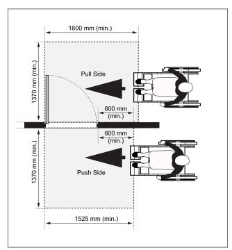
**Figure 41d:** Latch Side Approach at Side-Hinged Door - Plan View
