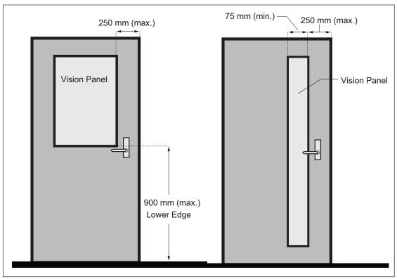
Figure 45: Vision Panels - Elevation View
