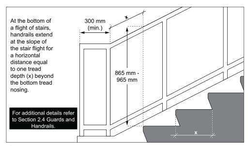
Figure 12: Handrail Extensions at Stairs - Section View
