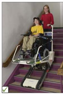
Example of portable elevating device, with platform designed to accommodate mobility aid during evacuation.
