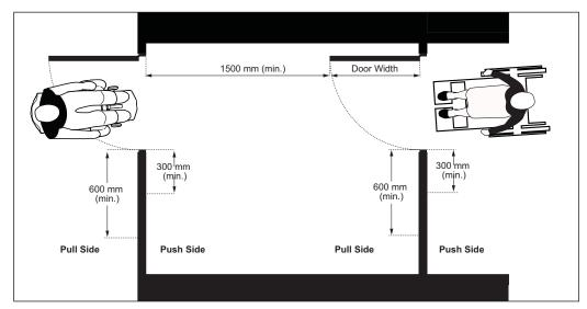
Figure 43: Doors in Series - Plan View
