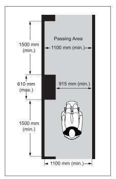
**Figure 46c:** Permitted Reduced Clear Width
