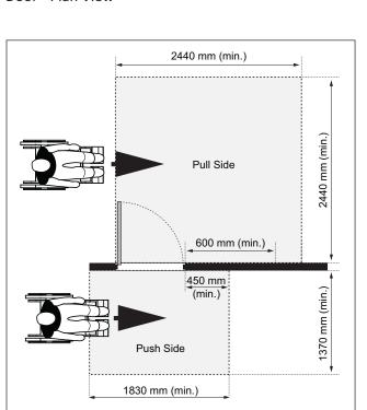
**Figure 41c:** Hinge Side Approach at Side-Hinged Door - Plan View
