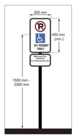
**Figure 25:** Accessible Parking Vertical Signage
