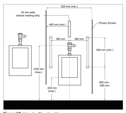
Figure 60: Urinals - Elevation View
