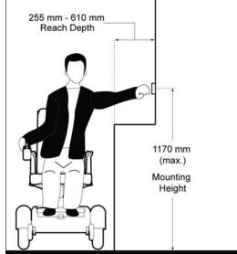
**Figure 66b:** Obstructed Side Approach and Reach: Depth 255 to 610 mm (Maximum)
