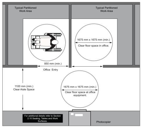
Figure 88: Common-Use Work Areas - Plan View
