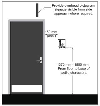
**Figure 70:** Mounting Height and Provisions of Permanent Signage - Elevation View
