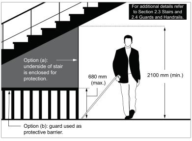
Figure 14: Protection Options Underneath Stairs
