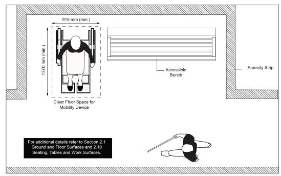
Figure 16: Rest Area - Plan View
