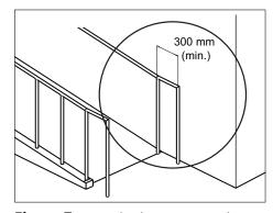
**Figure 7a:** Handrail Returns to Guard or Rail
